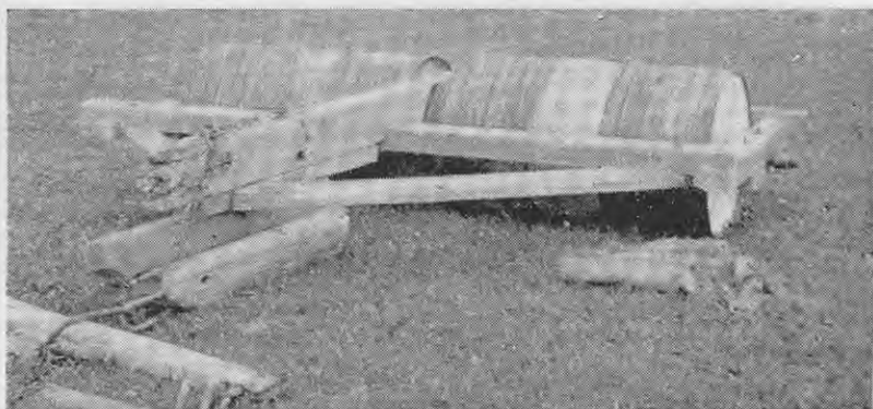
The roller described in this article. Note the provision made for a central bearing to prevent bending of the axle and the sledge foot in front to prevent "digging in."
