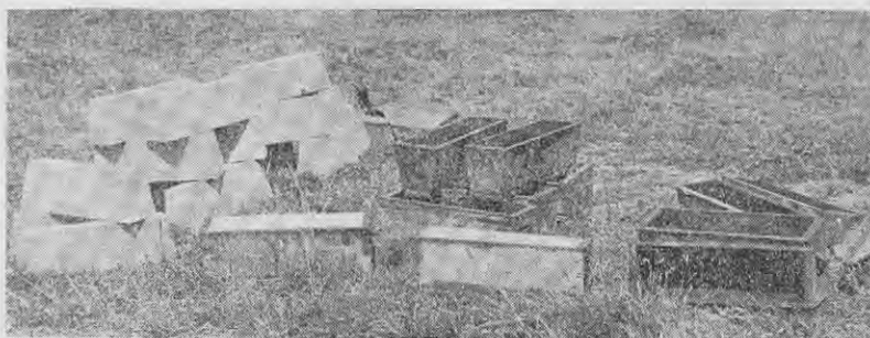
Concrete blocks and moulds. The blocks shown are used for supporting beehives, but may be used for a variety of other purposes.
