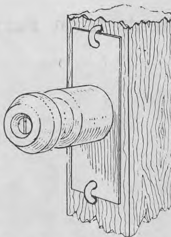
A rust-proof insulator fence-plate and insulator, which minimises breakages, faulty insulation and loss of power. The plates are fixed by driving a medium-sized fencing staple through each of the end holes. The insulator is then attached by a metal thread screw.
