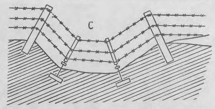
"To erect the fence, first put in the instead of around it, as in ordinary end posts which, as already mentioned, need only be good, solid, fencing posts. On firm ground staying is unnecessary, but they should be footed and crossbraced as shown in Fig. A. Sharp angles may be tied with a wire tie or braced like end-posts. A heavy post well rammed is sufficient for a slight angle. In placing an angle post it must be remembered that the wire will run some inches inside the post
