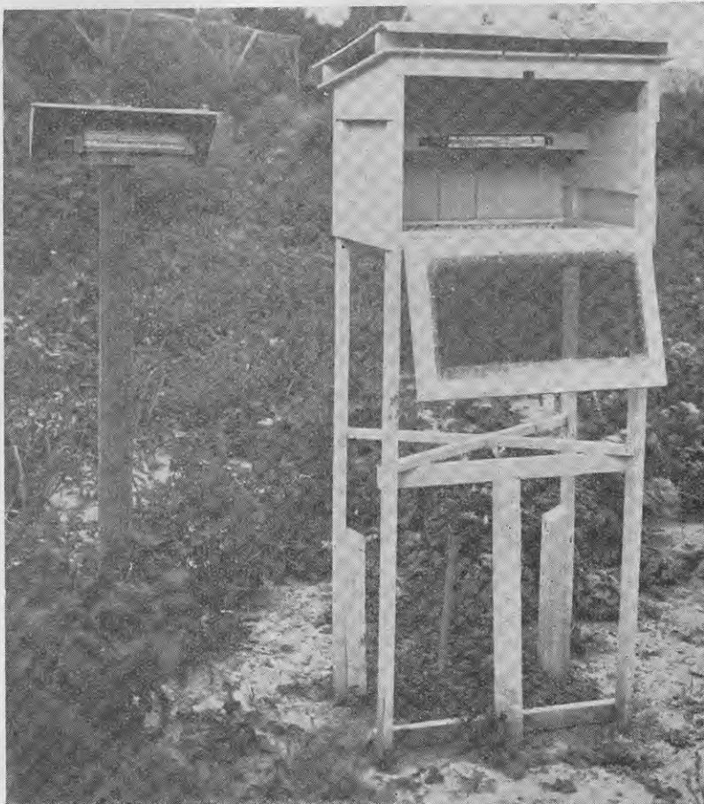
Two types of home-made orchard thermometer shelters. On the right is a standard type which is, perhaps, more carefully made than usual. On the left is the one commonly used in Central Otago; both back and top boards might with advantage have been a little larger.
