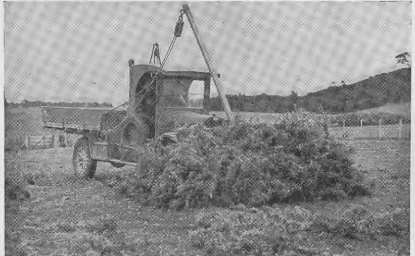
Fig. 2. —The sweep in operation clearing a paddock of grubbed gorse.
