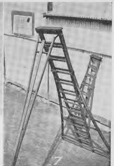
Fig. 5.—A 14 ft. ladder illustrating bent stays and clearance of legs from ground. The weight is taken by the stays, thus giving security on uneven ground.
