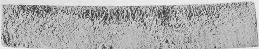
FIG. 9. TYPICAL DEPTH OF SAP-STAIN OCCURRING IN CLOSE-STACKED UNTREATED PILE.
