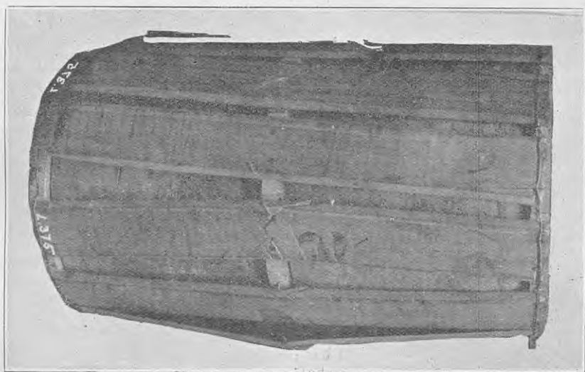
FIG. 10. TYPICAL FAILURE OF TWO-WIRED CRATE.
