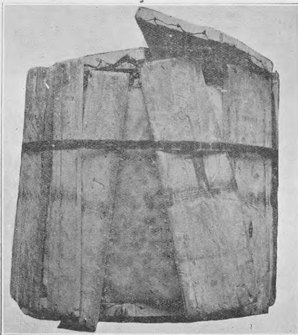
FIG. 14. TYPICAL FAILURE OF A CLEATED SINGLE-CHEESE CRATE.
