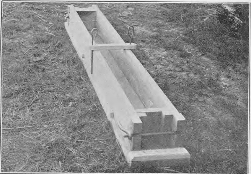
FIG. 6. MOULD SIMILAR TO THAT SHOWN IN FIG. 7 (SEE NEXT PAGE), BUT WITH CLEATS AND IRON PINS INSTEAD OF DOWELS.
