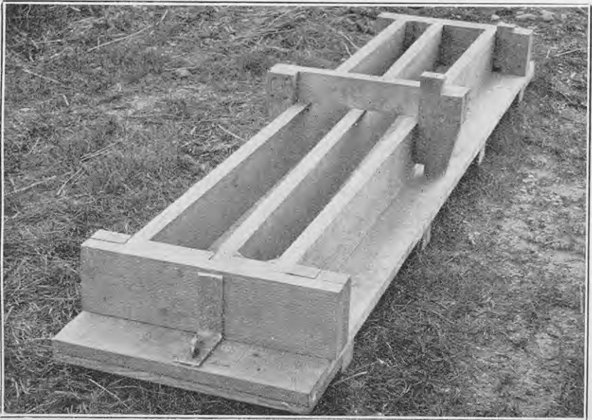
FIG. 5. TWO-POST MOULD OF SIMILAR DESIGN TO THAT GIVEN FOR THE FOUR-POST MOULD (FIG. 4).
