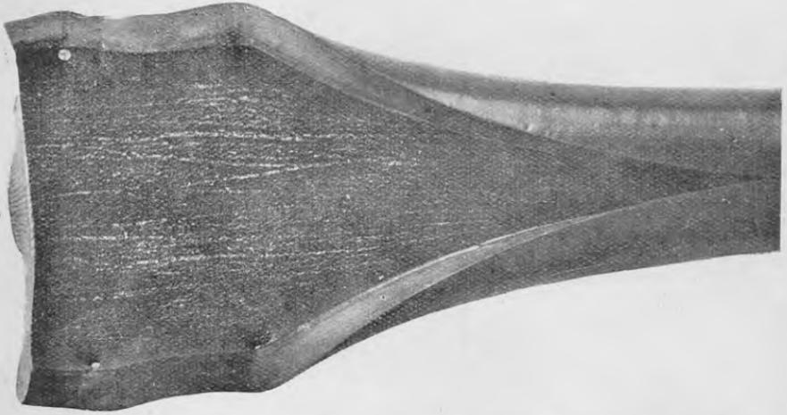
FIG. 1. LONG MILK-RUBBER AFTER TWELVE MONTHS' USE AND CLEANING DAILY WITH BOILING WATER, WASHING-SODA, AND THE USE OF A BRUSH AND SCRAPER. NOTE THE SCORED INNER SURFACE OF THE TUBE.
