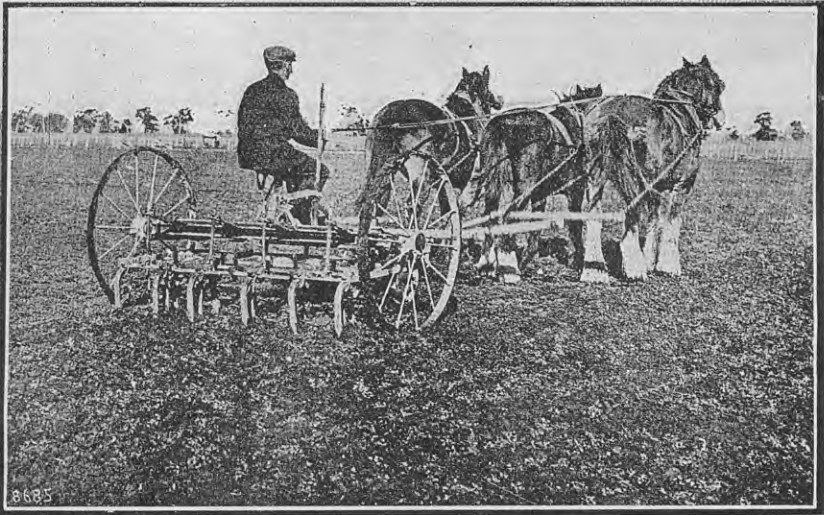
RENOVATING A LUCERNE-FIELD IN AUSTRALIA WITH THE SUNSHINE RIGID-TINE CULTIVATOR.
